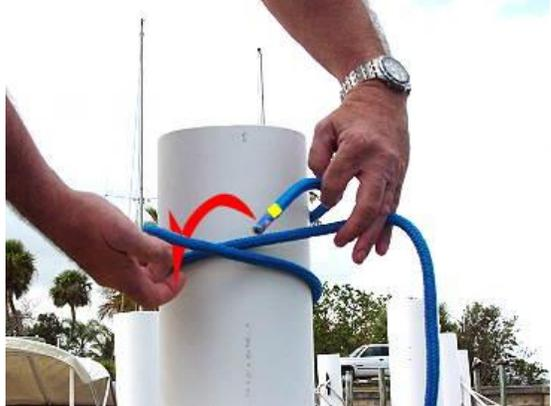
**Two Half Hitches** ~ may be used for securing a fender, or a tying a line to a piling
